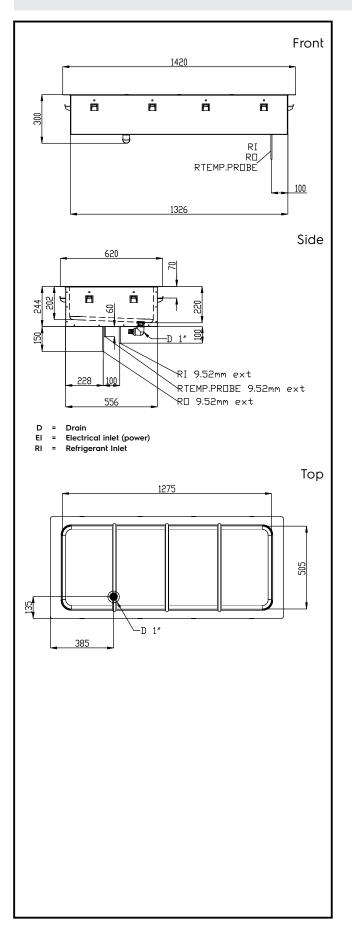
Drop-In Drop-in remote refrigerated well, static (4 GN container capacity)
